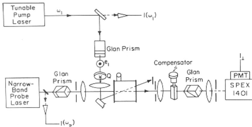
**Figure 7.** (from reference [27]) Typical RIKES experimental setup.
